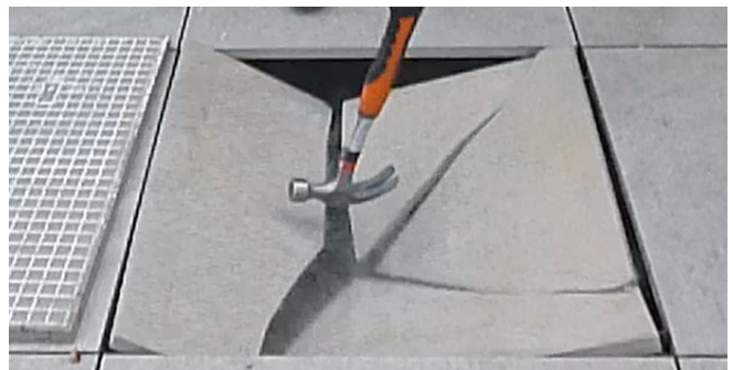
Photo 4. Screen shot from a video where I was able to break a 20mm porcelain tile dropping a 906g (2lbs) claw hammer from 600mm).
