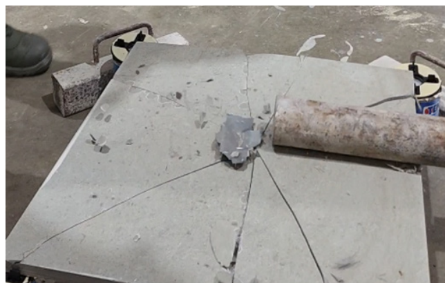
Photo 5. Tile fractured on pedestals, reinforced with a fiberglass matting adhered with cementitious adhesive. Load used to break the tile was a 10kg steel weight with a diameter of 60mm.
